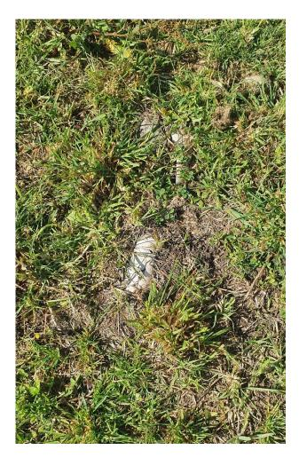
Image 6 Broken PVC pipe in surface soils
